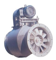
MK Axial Flow Fans are made from heavy gauge mild steel sheets, roll formed & welded. Impellers are either fixed or adjustable pitch in cast aluminium construction. Different type of drive arrangement are available i.e. A) Direct B) V - Belt C) Bifurcated.
